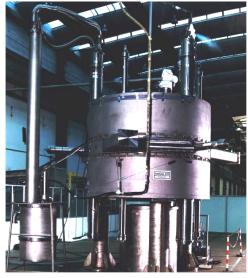
AGOR cryostat during factory cold test
