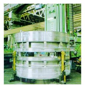
Machining of the cold mass after seal welding
